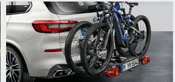
○ The BMW Pro 2.0 rear bicycle rack is lightweight yet sturdy and can carry up to 60 kg. Exceptionally easy to use, it carries two bicycles or e-bikes (can be extended to accommodate three bicycles). Its tilt function also allows easy access to the luggage compartment at all times.
