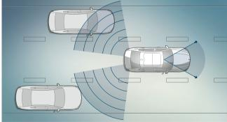
■ At speeds of over 70 km/h, Lane Departure Warning<sup>2</sup> recognises lane markings and draws the driver's attention to an unintentional lane change by means of vibration in the steering wheel. If a vehicle enters the driver's blind spot, **Lane Change Warning**<sup>1</sup> alerts the driver with a vibration in the steering wheel and a blinking symbol on the wing mirror.
