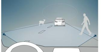
☐ **BMW Night Vision** with person recognition makes people and large animals visible on the Control Display from a distance using heat imaging and illuminates them with the Dynamic Marker Light in the main headlight. An additional warning system is also automatically activated when the vehicle is started, regardless of the status of the imaging display.
