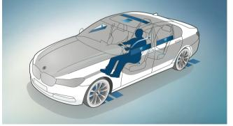
■ Active Protection warns the driver if it detects signs of tiredness, intervenes in critical situations and brakes the car to a standstill after an accident.
