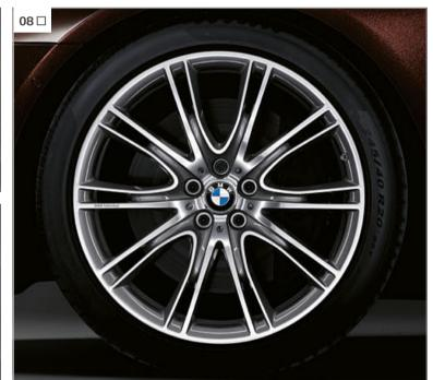
[ 01 ] 20" light alloy wheels V-spoke style 6281, Bicolour, with mixed tyres and runflat properties. Front: 8.5 J x 20 with 245/40 R 20 tyres. Rear: 10 J x 20 with 275/35 R 20 tyres.
