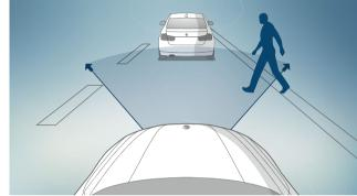
■ While Approach control warning with full city **braking** detects vehicles, **Pedestrian warning** reacts to people in the road. At the same time, the brakes are pre-conditioned for faster responsiveness. If a collision is imminent, the system initiates full braking.
