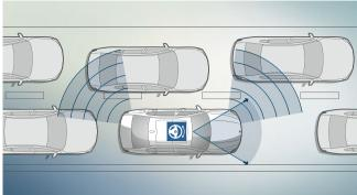
☐ Driving Assistant Plus includes **Lane Keeping assistant** with active side collision protection. This actively intervenes in steering to prevent the vehicle from leaving the lane unintentionally, or colliding with objects to the side of the vehicle.
