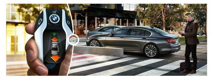
The **Remote Control Parking¹** function allows the driver to conveniently step out of the vehicle and use the remote control to move it forward into a tight space or garage or to reverse park. The driver activates the remote-controlledparking function from outside the vehicle via the standard BMW Display Key.
