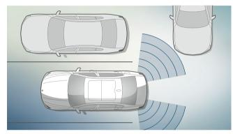
■ Crossing-traffic warning, rear, and Rear collision **prevention** from the Driving Assistant warns of approaching traffic when visibility is poor and detects the threat of a collision. Warning indicators alert following traffic of a potential impact.
