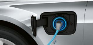
■ The vehicle can be charged from household power sockets with the charging cable supplied or on the go at public charging stations with a cable available from BMW Accessories. The navigation system and the BMW ConnectedDrive app inform the driver of the location and availability of stations where charging can take place, for example, with the ChargeNow card.
