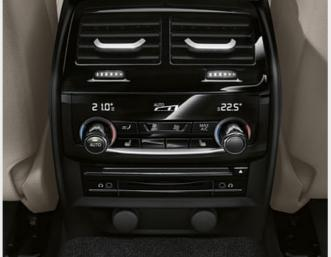
☐ The Automatic air conditioning with 4-zone control comes with the equipment included in Automatic air conditioning with 2-zone control with extended features, along with two air vents in the B columns. Additionally, the rear passengers can individually adjust their own climate via a separate control element with display.
