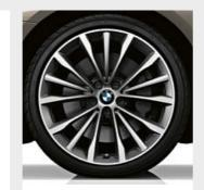
☐ 19" light alloy wheels W-spoke style 663 Ferric Grey gloss-lathed with mixed tyres and run-flat properties, front 8J x 19 with 245/40 R19 tyres, rear 9J x 19 with 275/35 R19 tvres.
