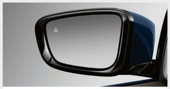
☐ If the indicator is on, the radar-based Lane Change Warning² warns the driver to approaching vehicles in the blind spot as well as vehicles in the neighbouring lane. The system functions beginning at speeds of 20 km/h, and in dangerous situations, it causes the steering wheel to vibrate and the triangle symbol in the exterior mirror to blink.
