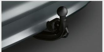
☐ The trailer tow hitch with electrically adjustable tow ball is approved for heavy loads of up to 2,000 kg. In order to stabilise things, trailer stability control automatically brakes the pulling vehicle if the trailer begins to swing. The electronically adjustable tow ball is not visible when stowed under the
