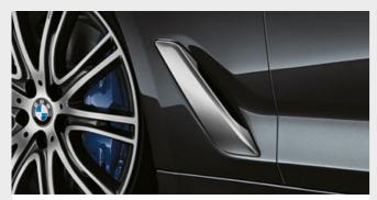
■ The Air Breather channels air to the front wheels, reducing air resistance, fuel consumption and CO<sub>2</sub> emissions.
