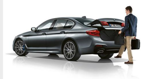
☐ Automatic tailgate operation allows the convenient opening and closing of the tailgate by simply pressing the conveniently located button in the door panelling or on the car key. The tailgate can also be opened in the conventional manner, using the outside handle, and closed using a button on the inside of the tailgate.
