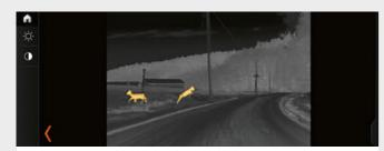
☐ BMW Night Vision¹ with person recognition makes people and large animals visible on the Control Display from a distance using heat imaging and illuminates them with the Dynamic Marker Light in the main headlight. An additional warning system is also automatically activated when the vehicle is started, regardless of the status of the imaging display.
