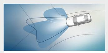
☐ LED headlights with Adaptive headlights, variable city and motorway light distribution and BMW Selective Beam provide optimum illumination of the road when driving in the dark. Even at a standstill, the integrated cornering lights are automatically activated by signalling or turning the steering wheel and are active at speeds of up to 35 km/h.
