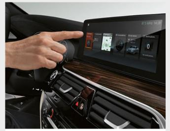
☐ With BMW Gesture Control<sup>1</sup>, certain functions can be operated by means of defined hand movements. For certain operations the system will for example recognise gestures such as 'swiping' or 'pointing' for accepting or rejecting an incoming call, or circular motions of the index finger to adjust volume.
