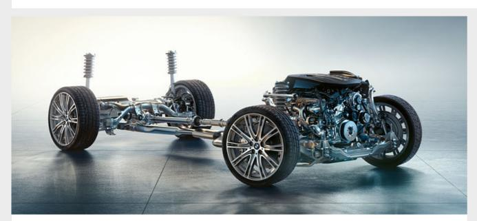
**Integral Active Steering**<sup>1,5</sup> combines support that varies based on the steering angle on the front axle, and rear wheels that also contribute to steering. At lower speeds, it offers greater manoeuvrability and agility by turning the rear wheels opposite the front wheels. Beginning around 60 km/h, the rear wheels turn parallel to the front wheels, to increase driving stability and comfort.
