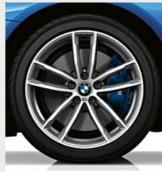
■ 18" M light alloy wheels Double-spoke style 662 M in Bicolour Ferric Grey gloss-lathed, with mixed tyres and run-flat properties, front 8J x 18 with 245/45 R18 tyres, rear 9J x 18 with 275/40 R18 tyres.
