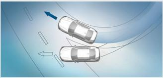
■ Dynamic Stability Control (DSC) permanently assesses the vehicle's movements and stabilises it using engine and braking regulation when unstable driving conditions are detected. Additional features of DSC are, for example, brake drying, braking readiness or the Hill-Start assistant, which holds the vehicle briefly in place when starting on inclines to prevent it from rolling backwards.
