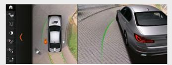
☐ The equipment package Parking Assistant Plus<sup>7</sup> makes parking and manoeuvring the vehicle easier. It features Surround View including Top View, Remote 3D View, PDC and the Parking Assistant with linear guidance, which parks the vehicle parallel or perpendicular to the lane completely automatically. The system works by measuring potential spaces while driving past them at a low speed.
