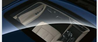
☐ The Glass roof with slide and lift function, including an electric sliding interior roof, anti-trap protection, as well as comfort opening and closing, allows the airflow to be individually regulated to create a pleasant interior climate. The integrated wind deflector prevents draughts from developing in the interior and ensures a lower level of wind noise.
